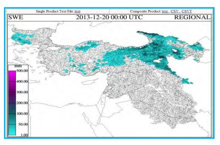
Snow Water Equivalent (SWE) product is a direct output of SNOW-17 accumulation and ablation model and estimated at 00, 06,12 and 18 UTC. SNOW-17 model gets two parameters namely GMAT and merged MAP and produces a number of products including SWE and MELT by using thermodynamic equations.
