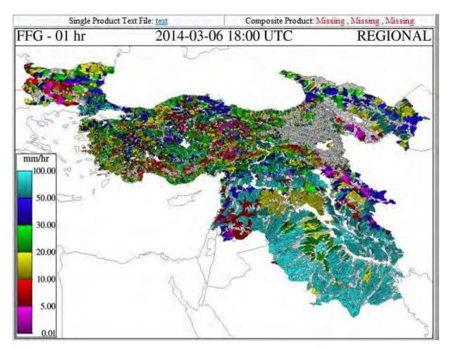
Flash Flood Guidance, which is defined as the amount of actual rainfall that causes bankfull flow at the end of catchment for a given duration e.g. 1,3 and 6 hours.
