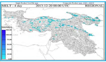
MELT is an estimate of ablation due to melt processes and is a direct output of SNOW-17 model. MELT is estimated every six hours at the model runtimes. 24-Hours and 96-Hour cumulative melt products are created from 6 hourly estimations.
