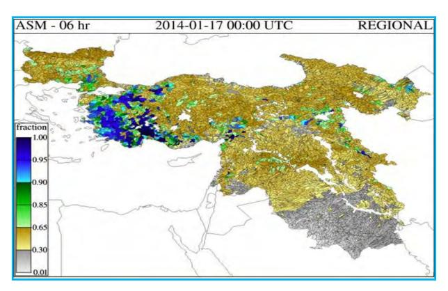
Average Soil Moisture (ASM) product shows fraction of soil moisture deficit of the upper soil (20-30 cm) for which upper zone tension and free water contents are estimated by using Sacramento Soil Moisture Accounting Model (SC-SMA).
