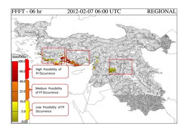
FFFT is the differences between forecast mean areal precipitation (FMAP) and FFG.
